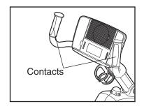
heart rate, hold the handgrip pulse sensor, with your palms resting against the metal contacts. Avoid moving your hands or gripping the contacts tightly.
